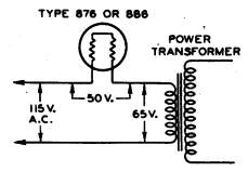
NOTE: THÈSE TUBES OPERATE AT A HIGH BULB TEMPERATURE AND MUST BE SURROUNDED BY A METAL VENTILATING STACK
