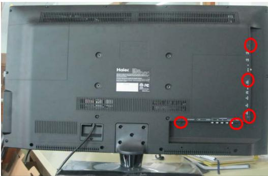
4-5. Remove the 2 screws fixing the socket connecting board
