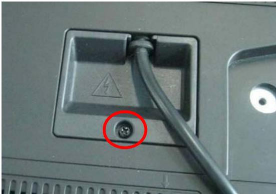
4-4.Remove the 9 screws on the back cabinet.
