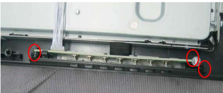
4-9.Remove the 2 screws fixing the remote sensor.
