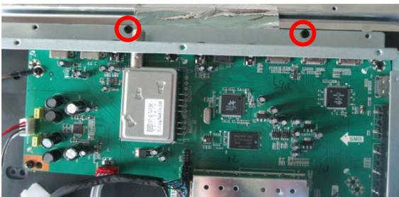
4-6.Remove the 6 screws fixing the main board
