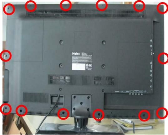
4-3.Remove the screw of the fixing board on the back cabinet.
