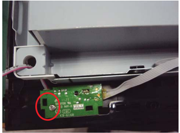
Remove the screw, take out the remote control board
