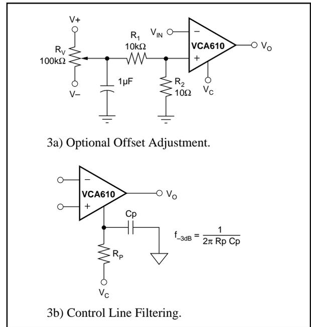
FIGURE 3. Optional Offset Adjustment and Control Line Filtering.
