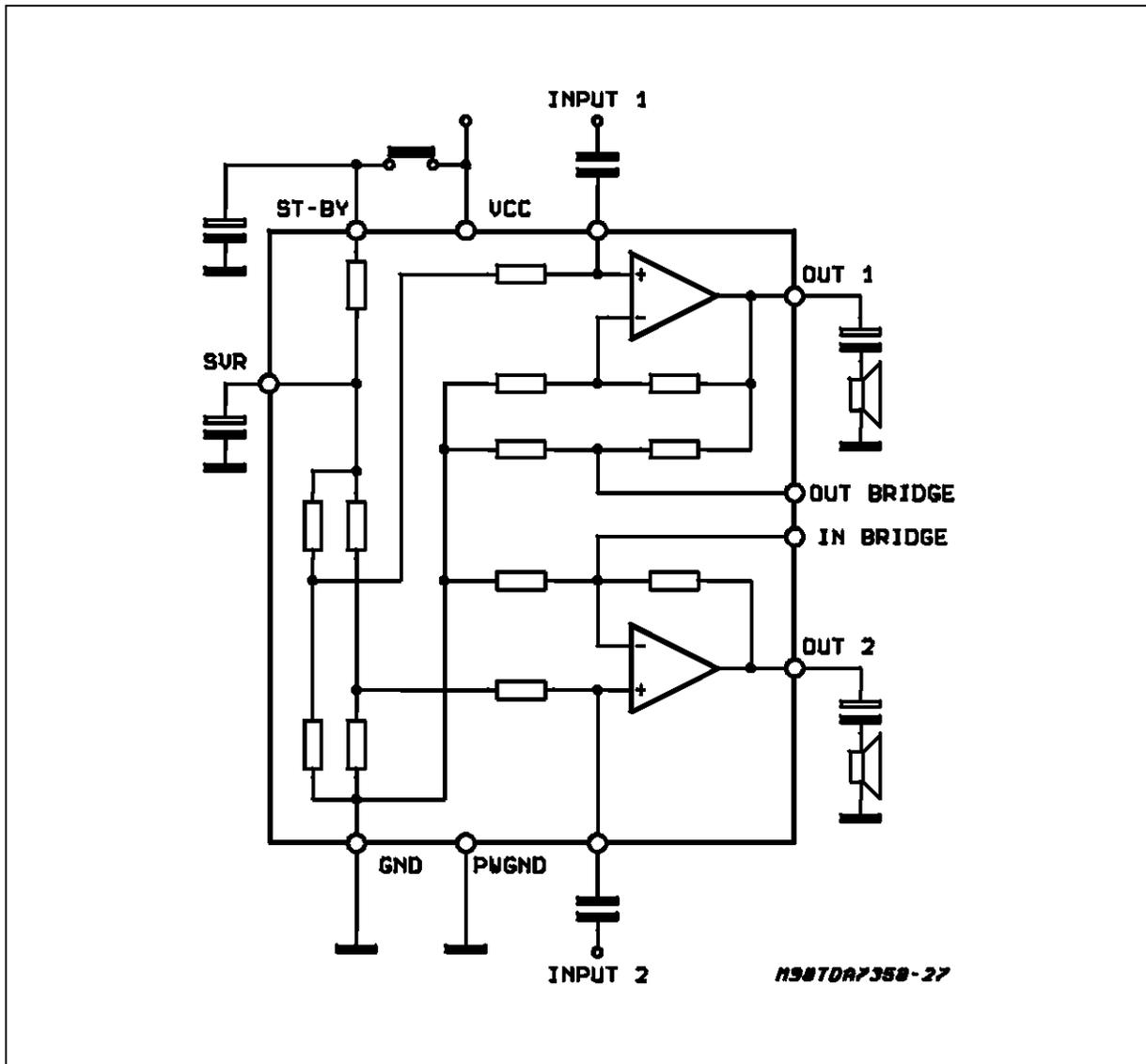
Figure 25: Turn-on Delay Circuit
