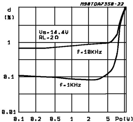
**Figure 14:** Distortion vs Output Power (Bridge)
