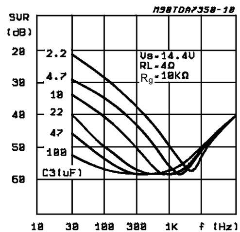
Figure 19: Crosstalk vs. Frequency (Stereo)
