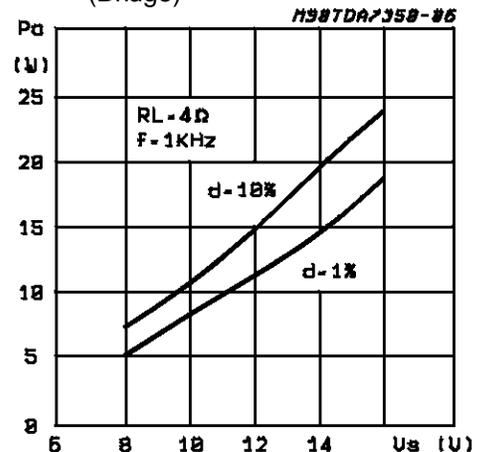
**Figure 9:** Output Power vs. Supply Voltage (Bridge)
