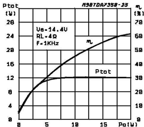
**Figure 23:** Power Dissipation & Efficiency vs. Output Power (Bridge)
