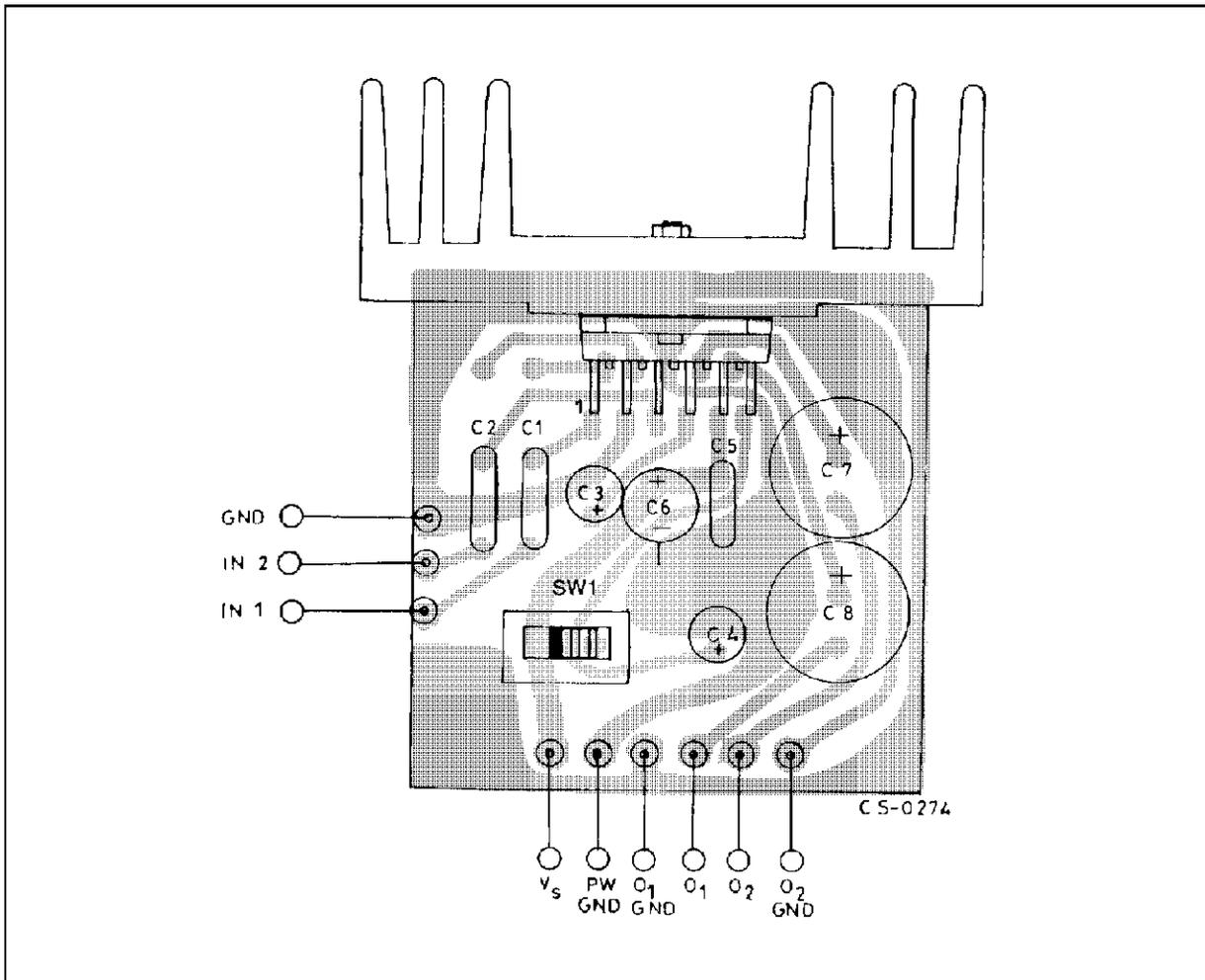
Figure 3: BRIDGE Test and Application Circuit
