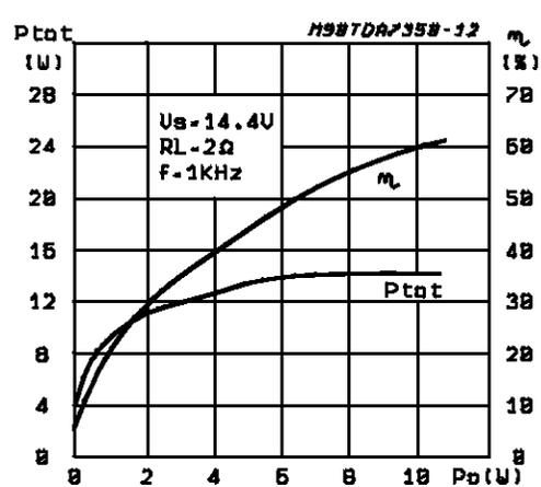
**Figure 21:** Power Dissipation & Efficiency vs. Output Power (Stereo)
