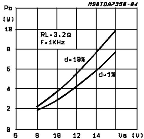
Figure 8: Output Power vs. Supply Voltage (Bridge)
