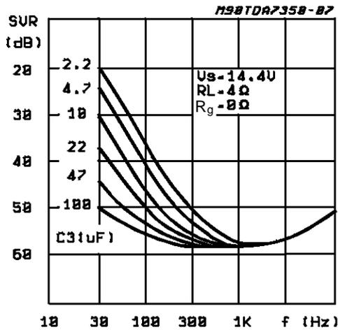
Figure 16: SVR vs. Frequency & C<sub>SVR</sub>; (Stereo)
