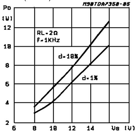
Figure 6: Output Power vs. Supply Voltage (Stereo)
