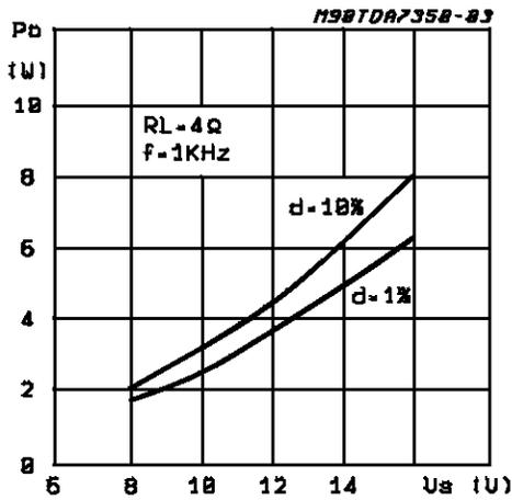
Figure 7: Output Power vs. Supply Voltage (Stereo)
