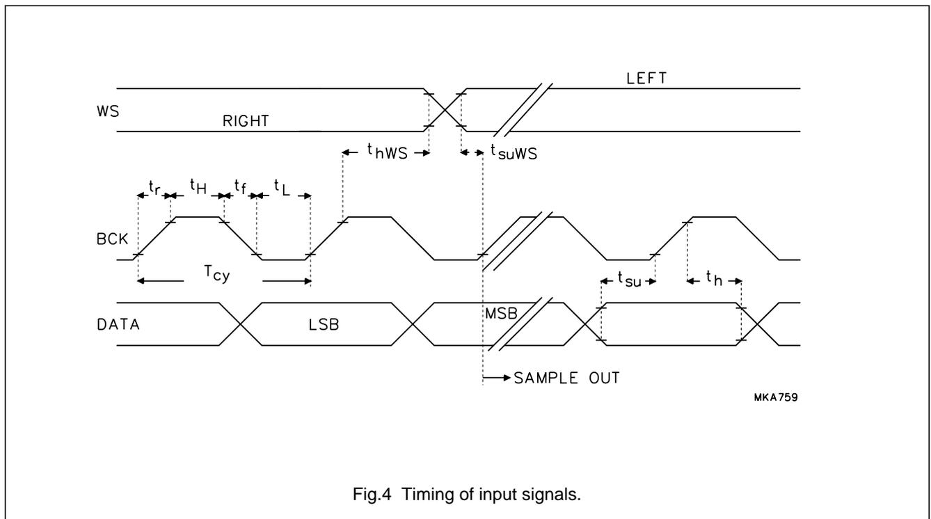
Fig.4 Timing of input signals.
