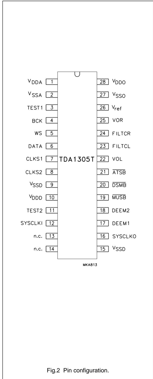
Fig.2 Pin configuration.
