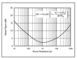
FIGURE 8. Noise Figure vs Source Resistance.
