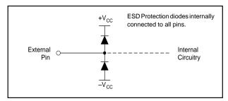
FIGURE 2. Internal ESD Protection.
