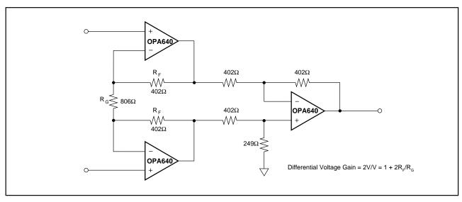
FIGURE 14. Wideband, Fast-Settling Instrumentation Amplifier.
