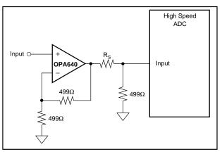
FIGURE 10. Differential Input Buffer Amplifier (G = +2V/V).
