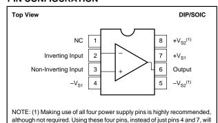
lower the effective pin impedance and substantially lower distortion.
