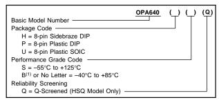
NOTE: (1) The "B" grade of the SOIC package will be designated with a dot. Refer to the mechanical section for the location.
