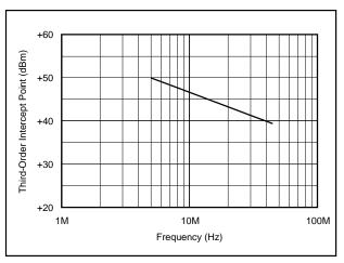
FIGURE 7. Single-Tone , 3rd-Order Intercept Point vs Frequency.
