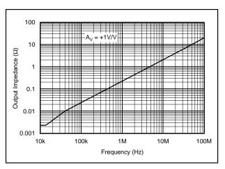
FIGURE 3. Closed-Loop Output Impedance vs Frequency.
