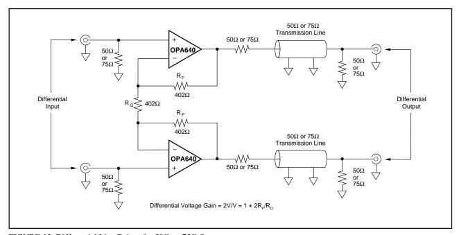
FIGURE 13. Differential Line Driver for  $50\Omega$  or  $75\Omega$  Systems.
