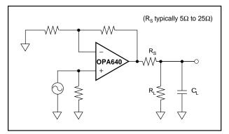
FIGURE 5. Driving Capacitive Loads.
