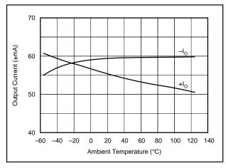
FIGURE 4. Output Current vs. Temperature.
