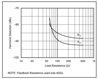
FIGURE 6. 5MHz Harmonic Distortion vs Load Resistance.
