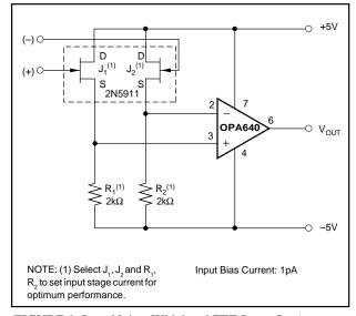
FIGURE 9. Low Noise, Wideband FET Input Op Amp.
