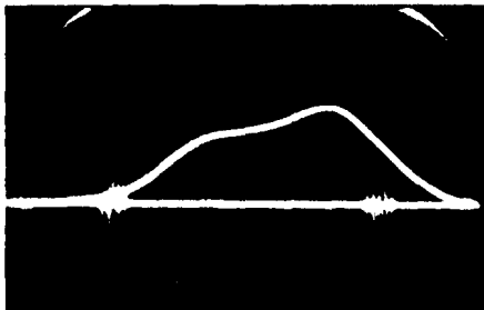
Figure 12. Band Pass Displayed by Conventional Sweep
