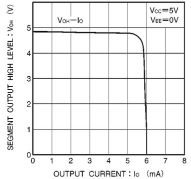
Fig. 8 Segment high level output vs. output current
