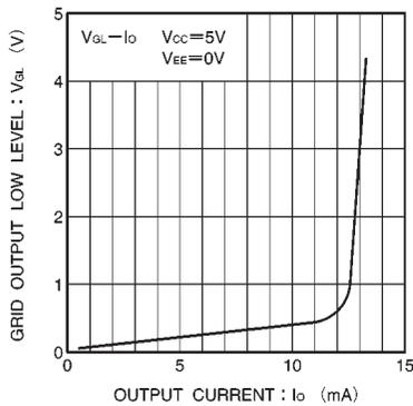
Fig. 9 Grid lowlevel output vs. output current
