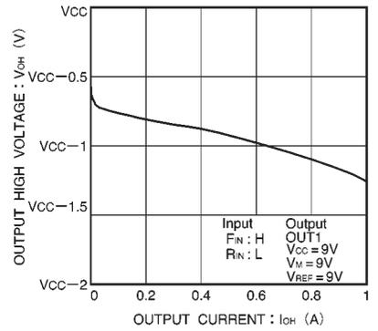
Fig.5 Output high level voltage vs. output current
