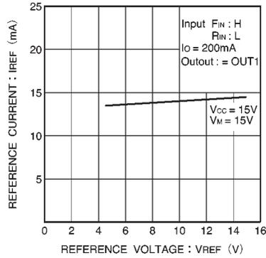
Fig.7  $V_{REF}$  reference current vs.  $V_{REF}$  reference voltage
