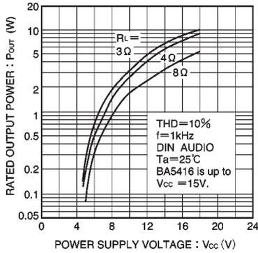
Fig. 16 Rated output voltage vs. power supply voltage
