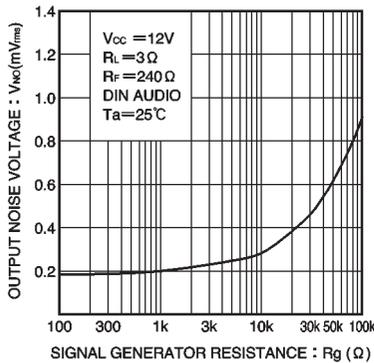
Fig. 19 Output noise voltage vs. signal source resistance
