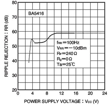
Fig. 24 Ripple rejection vs. power supply voltage (BA5416)
