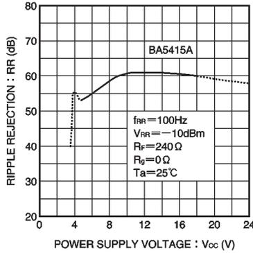
Fig. 23 Ripple rejection vs. power supply voltage (BA5415A)
