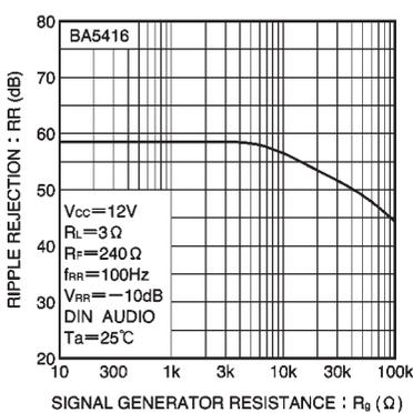
Fig. 28 Ripple rejection vs. signal source resistance (BA5416)
