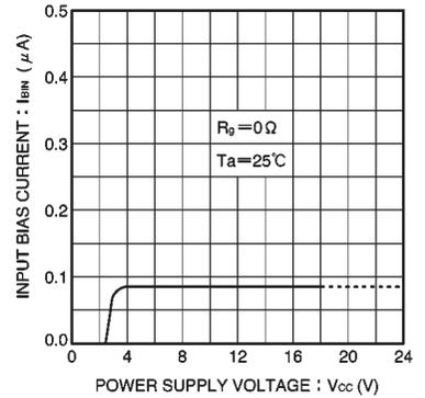
Fig. 18 Input bias current vs. power supply voltage
