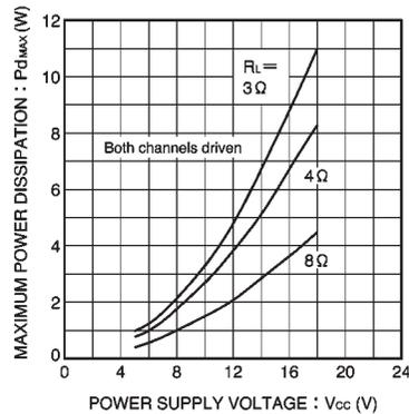
Fig. 29 Maximum power dissipation vs. power supply voltage
