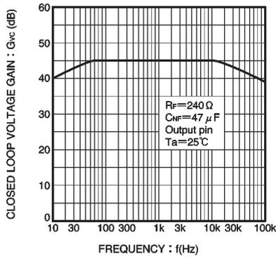
Fig. 13 Closed loop voltage gain vs. frequency
