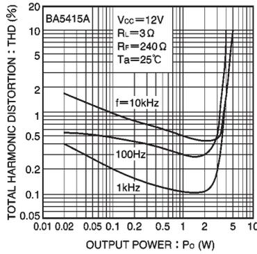
Fig. 14 Total harmonic distortion vs. output power (BA5415A)
