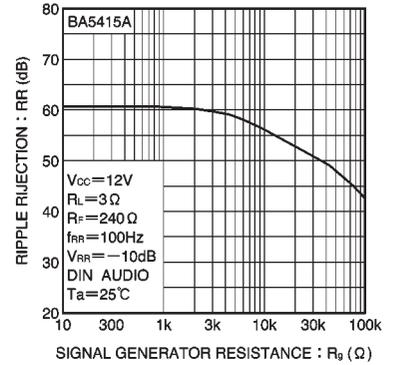
Fig. 27 Ripple rejection vs. signal source resistance (BA5415A)
