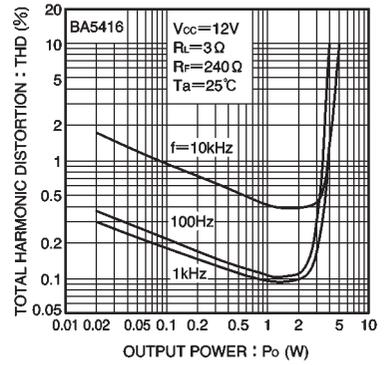
Fig. 15 Total harmonic distortion vs. output power (BA5416)
