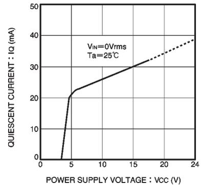
Fig. 12 Quiescent current vs. power supply voltage
