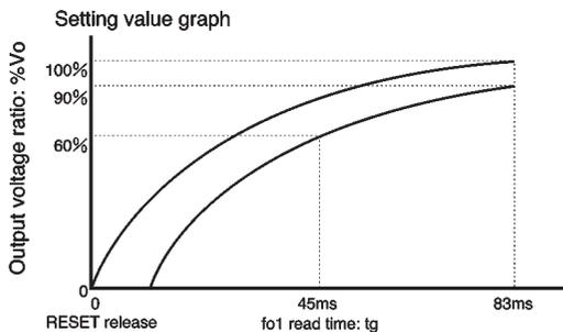
Fig. 7 fo1 read time vs. output voltage
