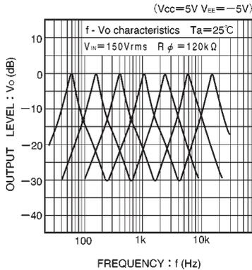
Fig. 10 Output level vs. frequency
