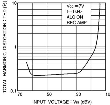
Fig. 9 Total harmonic distortion vs. input voltage
