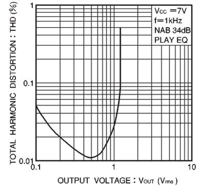
Fig. 10 Total harmonic distortion vs. output voltage
