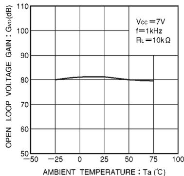
Fig. 12 Open loop voltage gain vs. ambient temperature
