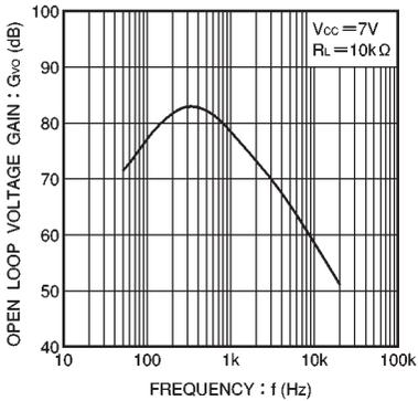
Fig. 8 Open loop voltage gain vs. signal frequency
