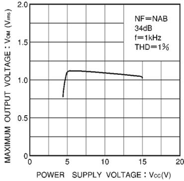
Fig. 6 Maximum output voltage vs. power supply voltage
