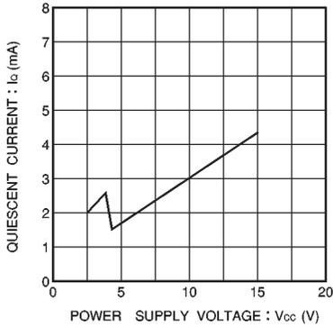
Fig. 5 Quiescent current vs. power supply voltage
